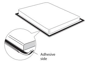
Fig. 4 Applying the adhesive seal around the edges of the cooktop
